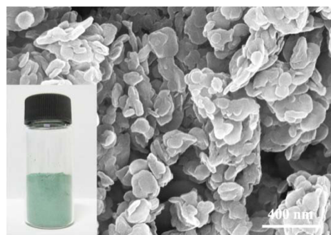
Figure 4. SEM image of the organic–inorganic \alpha\text{-Co}(\text{OH})_2 nanoplates intercalated with benzoate anions obtained by precipitation with NaOH. The inset is a photograph of the material.
