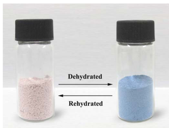
Figure 3. Photographs of \text{Co}(\text{OH})(\text{C}_6\text{H}_5\text{COO})\cdot\text{H}_2\text{O} nanofibers in (a) hydrated and (b) dehydrated forms. The nanofibers exhibit a reversible transformation of the coordination geometry of the \text{Co}^{\text{II}} ions between octahedral and pseudotetrahedral induced by heating at low temperature, which involves the loss and reuptake of unusual weakly coordinated water molecules without loss of crystallinity.
